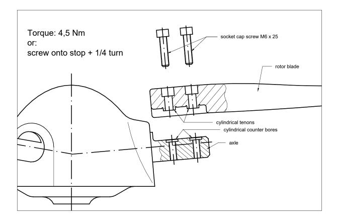
The rotor blades are fixed by two socket cap screws M6 x 25, which are TUFLOK-coated to prevent loosening at operation. When screwing in you will sense a slight drag torque due to the coating.
