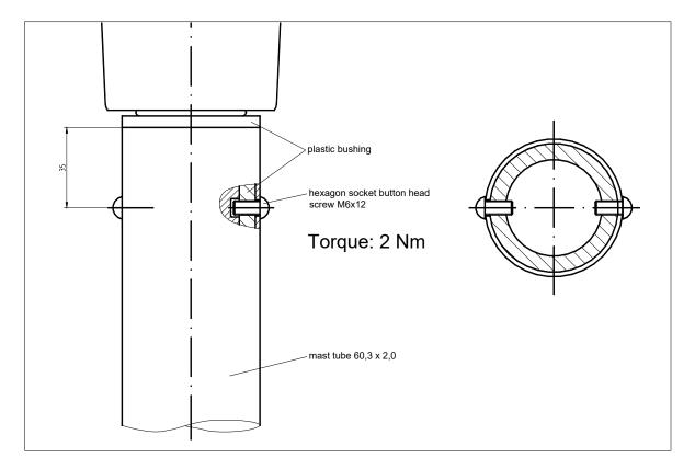
In the next drawing you can see that the two button head screws M6 x 12 protrude into the groove of the yaw shaft, but do not touch it. In order to ensure the function of the vibration and impact sound absorber, it is important that the two holes in the mast tube are carefully drilled.
